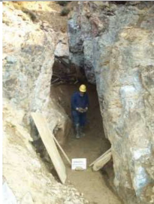
Removal of debris from the Dyffryn Coch adit. This may give access to early 18th century workings
